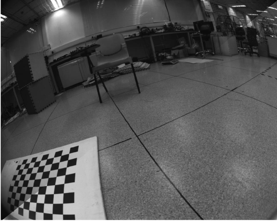
Figure 4.5: The demonstration of the vignetting. The top-left part is the raw image and the bottom-right part is removed vignetting.
